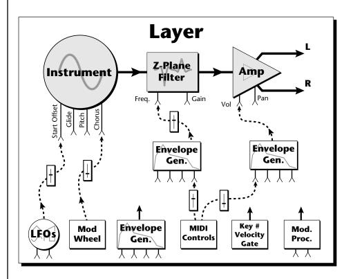
• Note-on modulation sources, such as key, velocity and gate output a single value at note-on time. Realtime modulation sources such as LFOs, envelope generators and modulation wheels can be varied continuously.
