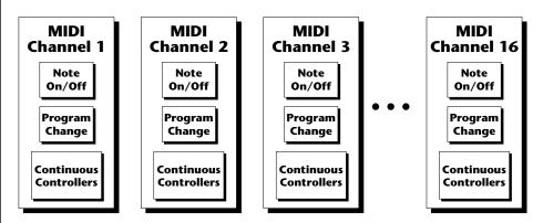
Any MIDI controller can be routed to any modulation destination. First, you have to know which controller numbers your keyboard transmits. Most modern MIDI keyboards let you select a controller number for each control on the keyboard. For example, it may let you select a number from 0-31 for the data slider. The realtime controller numbers that the keyboard transmits must match the numbers Virtuoso 2000 is receiving, otherwise nothing will happen when you move the controls.
