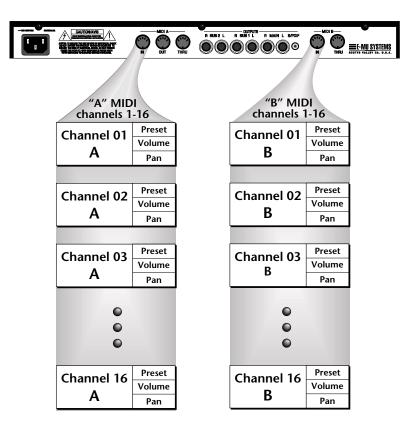
Virtuoso 2000 has two MIDI inputs with 16 MIDI channels each. Each of the 32 MIDI channels can be assigned to play a specific preset with unique volume and pan settings.
