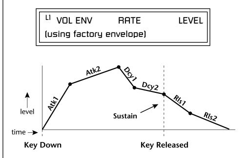
On the Volume Envelope, levels can only be set to positive values. The value range is from 0 to +100.
