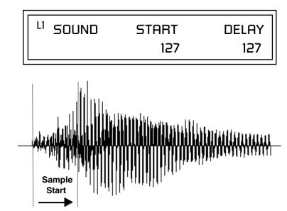
Controlling the Sound Start using Key Velocity (< Amt -) brings in the attack of the wave only when you play hard. This is especially effective with percussion instruments.
