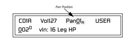
**Note:** Pan settings in the preset ADD algebraically with the Channel Pan setting. Therefore, if the pan setting in the preset were set to "63R," moving the Channel Pan setting full left would return the sound to the center position.
