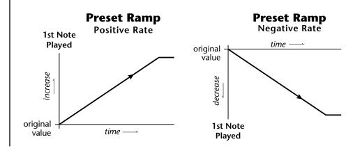
The preset ramp instantly resets when all notes have been released and the next *first key* on the MIDI channel is pressed. The Ramp Rate polarity (+ *or* -) determines if the ramp will be positive or negative going. The value of the ramp rate sets the increment. Large values produce fast ramps and small values produce slow ramps. Multiple inputs can be connected to the ramp rate (just like all the other destinations in Virtuoso 2000).
