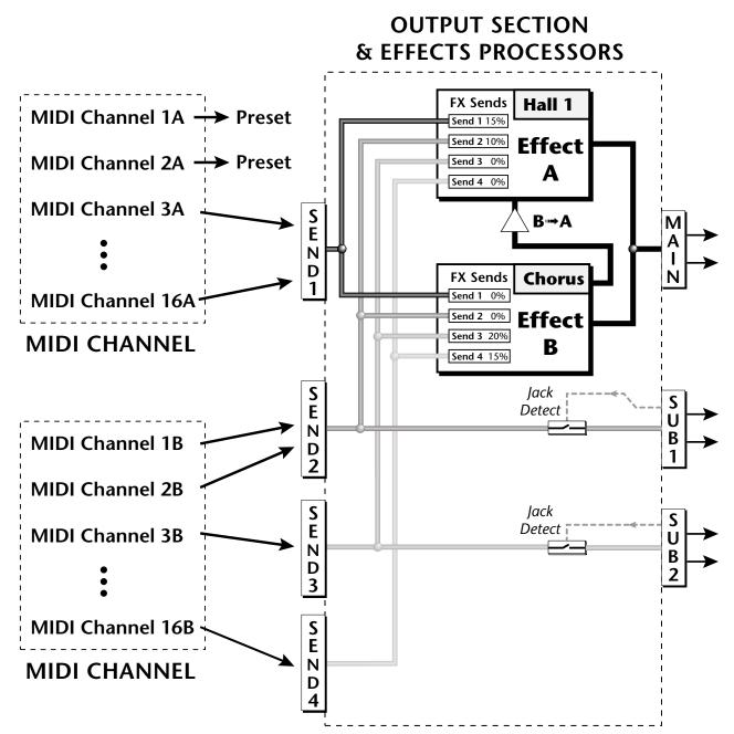
Sends 2 and 3 can be routed to the effects processors or to rear panel submix jacks. When a plug is inserted into a Submix jack, the dry portion of the Send is disconnected from the effects processor and is routed **directly** to the Submix output jacks.
