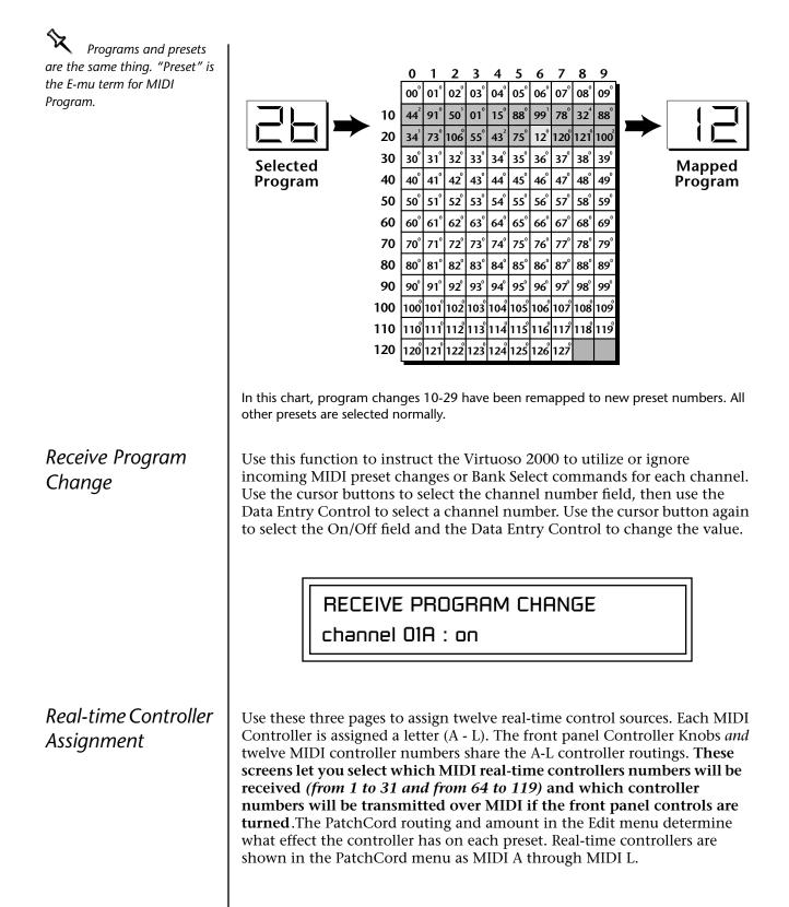
The Real-time Controller assignment also specifies which controller numbers are transmitted when the "Knobs MIDI Out" is enabled (see "Knobs/Riff MIDI Out" on page 51).
