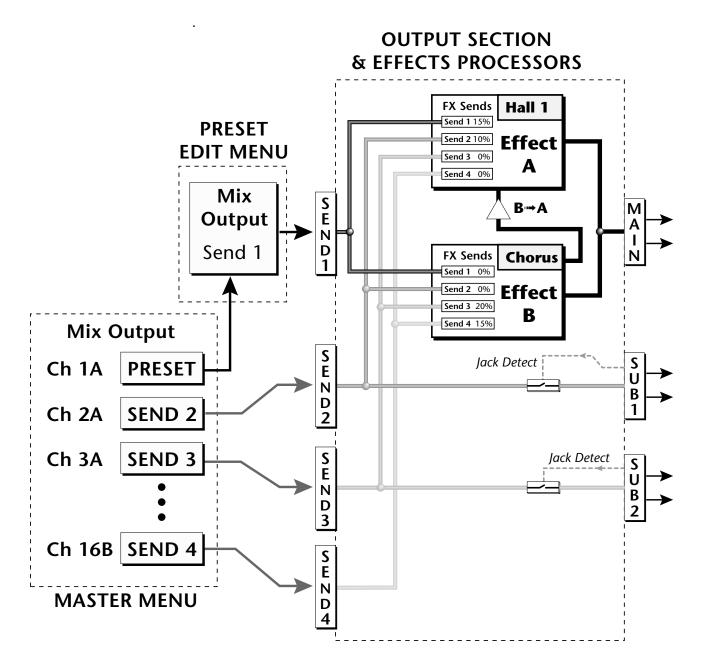
The Mix Output setting in the Master Menu determines if the Preset's Mix Output routing will be used. This allows the Sends to be programmed by either **MIDI Channel** or by **Preset**, whichever you prefer.
