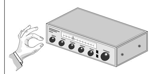
Turning the volume control back and forth on your home stereo is an example of Amplitude Modulation.
