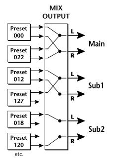
Each preset can be routed to one (and only one) set of stereo outputs. A preset can be routed to a single output using the pan control.
