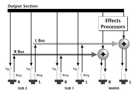
You can use the Sub 1 and Sub 2 jacks as effect returns to the Main Outputs. Note that the Effects Processors are only routed to the Main Outputs.
