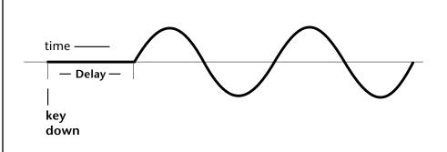
All Delay values equal to or greater than zero specify absolute time rates from 0 to 127. Values less than zero specify Tempo-based mode. Refer to the previous table for times and tempo-based rates.
