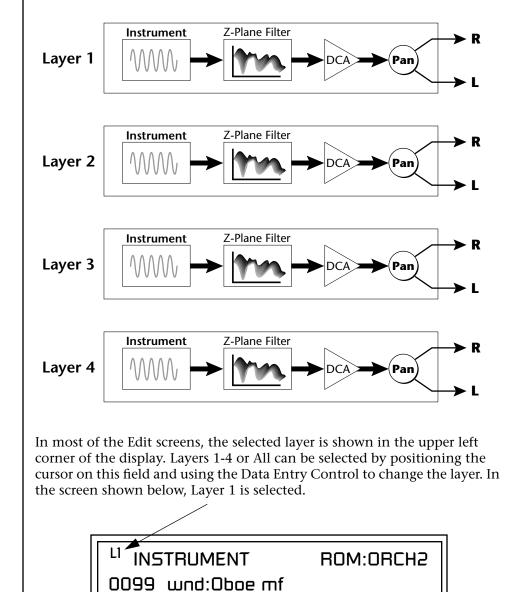
When "All Layers" (A) is selected, the existing parameter value for any field will be displayed if all layers are equal. If the layer parameter values are NOT equal, the value of Layer 1 will be displayed with flashing characters. If you move the Data Entry Control all values will be equal to this new value and the parameter value will no longer flash.
