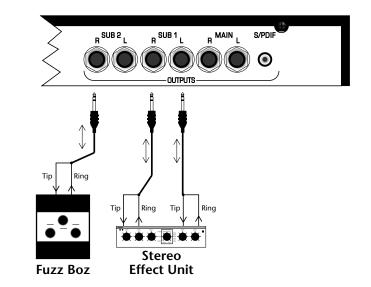
Using the submix outputs and returns, specific presets can be routed through your favorite effects without using up precious mixer channels.
