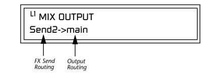
The entire Send is disconnected from the Effects Processors even if only one plug is inserted into the Submix jack.
