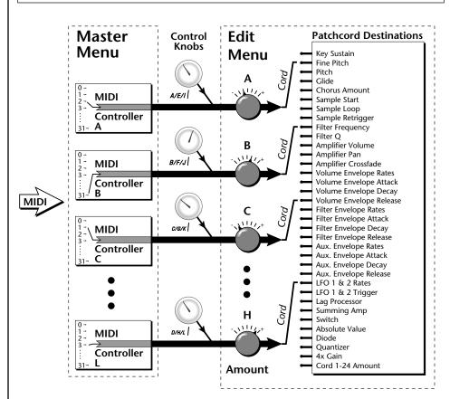
MIDI A-L are internal connections which simultaneously carry front panel controller knob data and MIDI continuous controller data.
